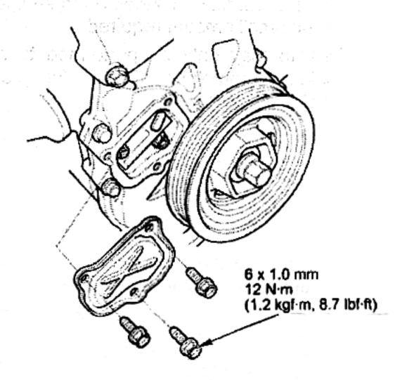
Reassemble in the reverse order of removal using new flange bolts torqued to the proper torque specs (12Nm, 8.7 lb-ft).
